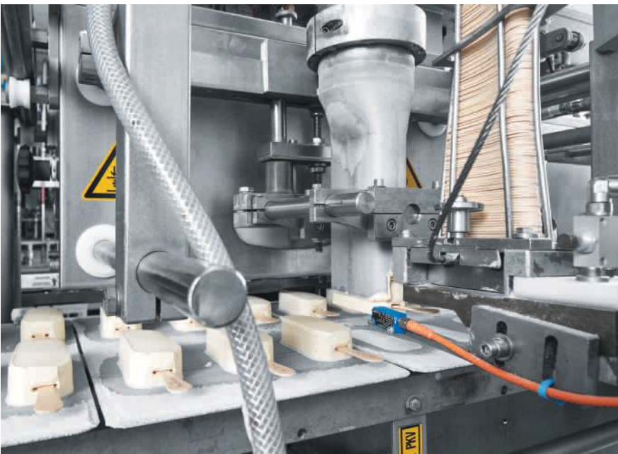
Perfectly portioned: the extruder outputs one Magnum core per second. The stick is inserted in the ice cream during extrusion.
