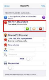
**Step 3:** Type in User ID and password. Then slide the button from disconnected to connected, which is highlighted in red below.
