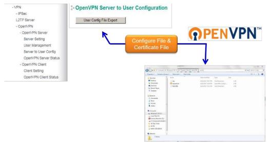
**Step 5:** Connect client to the server. Click the OpenVPN GUI icon. When OpenVPN connection is not built up, the icon will show in yellow.
