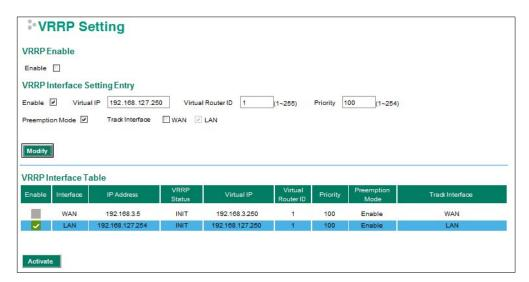
Virtual Router Redundancy Protocol (VRRP) can solve the problem with static configuration. VRRP enables a group of routers to form a single virtual router with a virtual IP address. The LAN clients can then be configured with the virtual router's virtual IP address as their default gateway. The virtual router is the combination of a group of routers, and is also known as a VRRP group.
