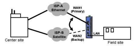
When configuring the EtherDevice Router, choose one of the two following conditions to activate the backup path:
