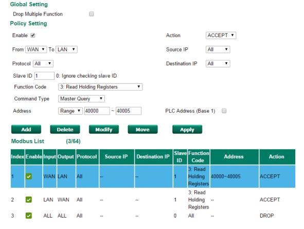
**Modbus TCP Filtering** controls both directions of communication between Modbus Master and Modbus Slave. Users need to set up two rules for the data transaction between Master and Slave. One rule is to accept the Master commands and another rule is to accept the Slave response.
