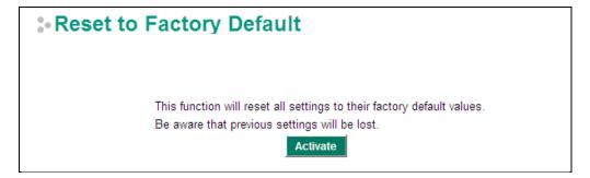
The **Reset to Factory Default** option gives users a quick way of restoring the EtherDevice Router's configuration settings to their factory default values. This function is available in the console utility (serial or Telnet), and web browser interface.
