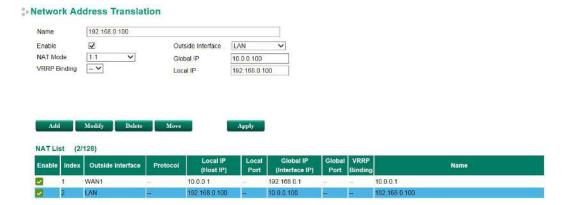
For some applications, devices need to talk to both internal devices and external devices without using a gateway. Bidirectional 1-to-1 NAT can do Network Address Translation in both directions without a gateway.
