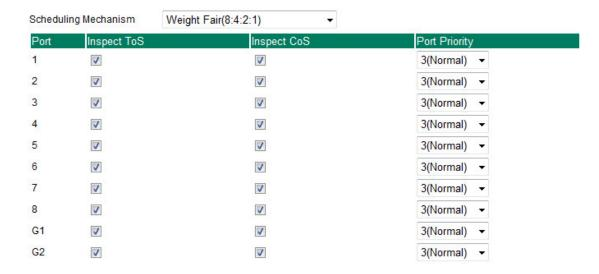
The Moxa switch supports inspection of layer 3 ToS and/or layer 2 CoS tag information to determine how to classify traffic packets.
