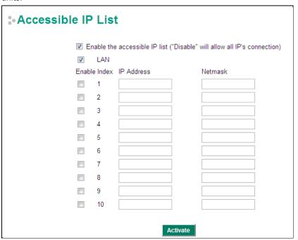
Accessible IP Settings allows you to add or remove "Legal" remote host IP addresses to prevent unauthorized access. Access to the EtherDevice Router is controlled by IP address. If a host's IP address is in the accessible IP table, then the host will have access to the EtherDevice Router. You can allow one of the following cases by setting this parameter:
