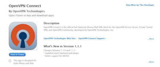
Step2: Download the ovpnclient.ovpn file from the Industrial Secure Router into the mobile device. And then open it with the OPenVPN. Connect App. Then the user will see the server IP, which is marked in red below. Then press "+"icon to add this VPN connection.
