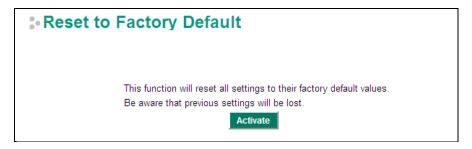
The **Reset to Factory Default** option gives users a quick way of restoring the Industrial Secure Router's configuration settings to the factory default values. This function is available in the console utility (serial or Telnet), and web browser interface.
