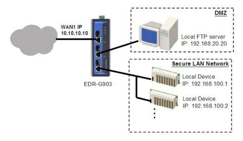
DMZ mode is configured on the **WAN2 configuration** web page. Set Connect Mode to Enable, Connect Type to Static IP, and checkmark the DMZ Enable check box. You will also need to input the IP Address and Subnet Mask. Click the **Activate** button to save the settings.
