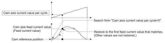
Search from a value in the middle of the cam axis current value per cycle. (Cam data starting point ≠ 0)
