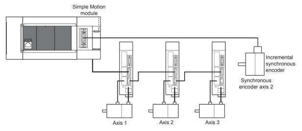
Set "1: Incremental synchronous encoder" in "[Pr.320] Synchronous encoder axis type" for the synchronous encoder axis 2. And, set the input method for incremental synchronous encoder signal in the following parameters.
