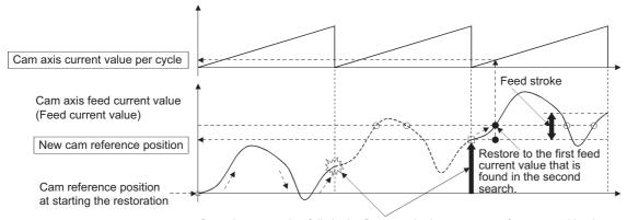
Once the restoration fails in the first search, the new cam reference position is automatically updated to set "Feed current value - New cam reference position" to be within the feed stroke amount, and the search process starts again.
