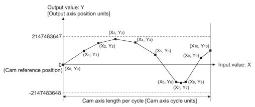
When an input value that is 0 or the cam axis length per cycle does not exist in the coordinate data, the coordinate is calculated from the line segment between the nearest two coordinates.
