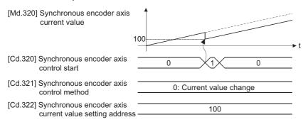
If set to "101 to 104", the synchronous encoder axis control starts based on the high-speed input request [DI] for the specified servo amplifier axis.
