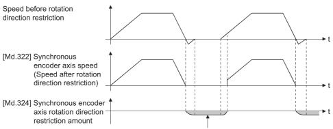
The input movement amount is accumulated as a rotation direction restricted amount, and will be reflected when the input movement amount moves in the enabled direction.
