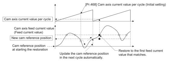
Search from a value in the middle of the cam axis current value per cycle. (Cam data starting point ≠ 0)
