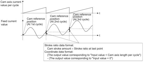
Create cam data for two-way cam operation as shown below.
