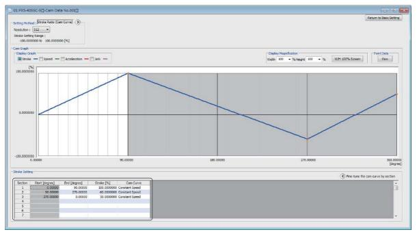
**4.** Set the synchronous parameter of the axis 1.
