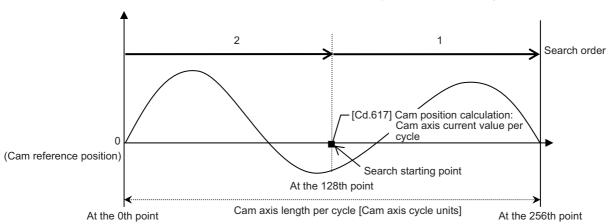
• Searches until between the 255th point and the 256th point (last point) in order of the cam data between the 128th point and the 129th point and between the 130th point and the 131th point.
