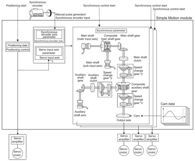
It is possible to control without amplifier by setting the virtual servo amplifier.
