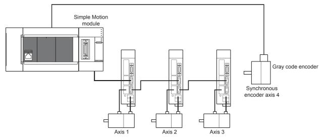
Set "201: Synchronous encoder via CPU" in "[Pr.320] Synchronous encoder axis type" of synchronous encoder axis 4. Set "4096" in "[Pr.329] Resolution of synchronous encoder via CPU" of synchronous encoder axis 4.
