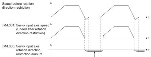
The input movement amount is accumulated as a rotation direction restricted amount, and will be reflected when the input movement amount in the enabled direction.
