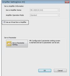
2. Set the axis 4 as the servo input axis in the input axis parameter.
