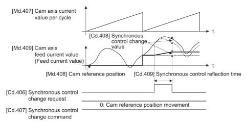
When "[Cd.406] Synchronous control change request" is reset to "0" while executing the cam reference position movement instruction, operation is stopped midway. If the cam reference position movement instruction is executed again, the remainder movement amount is not reflected, and the operation starts with "[Cd.408] Synchronous control change value" to be used again.
