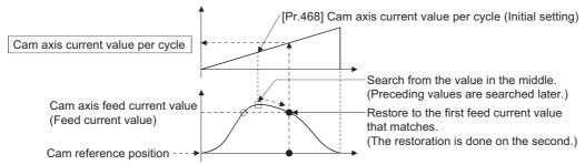
Search from a value in the middle of the cam axis current value per cycle. (Cam data starting point ≠ 0)
