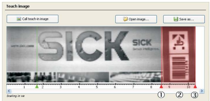
Fig. 36: Menu "Teach" – Window "Teach image" – Specify starting and end values by moving the red line with the mouse pointer.
