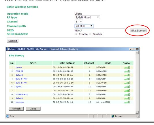
NOTE If the Gateway field in Basic Settings → Network Settings is empty, a warning message will appear, reminding you to set the default gateway when Client mode is enabled. You can ignore this message if you are only planning a local network and packets will not be sent outside the network.
