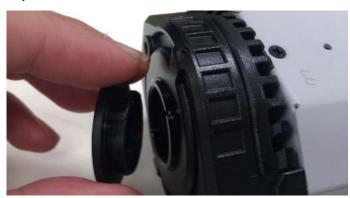
Step 2: Loosen the lens holder screw with the torx screwdriver.
