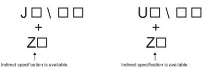
The access destination can be switched with one message, by changing the value of the index register in CPU module programs.
