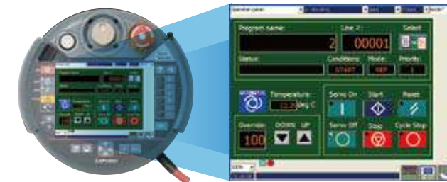
Robot control screen (R56TB)
