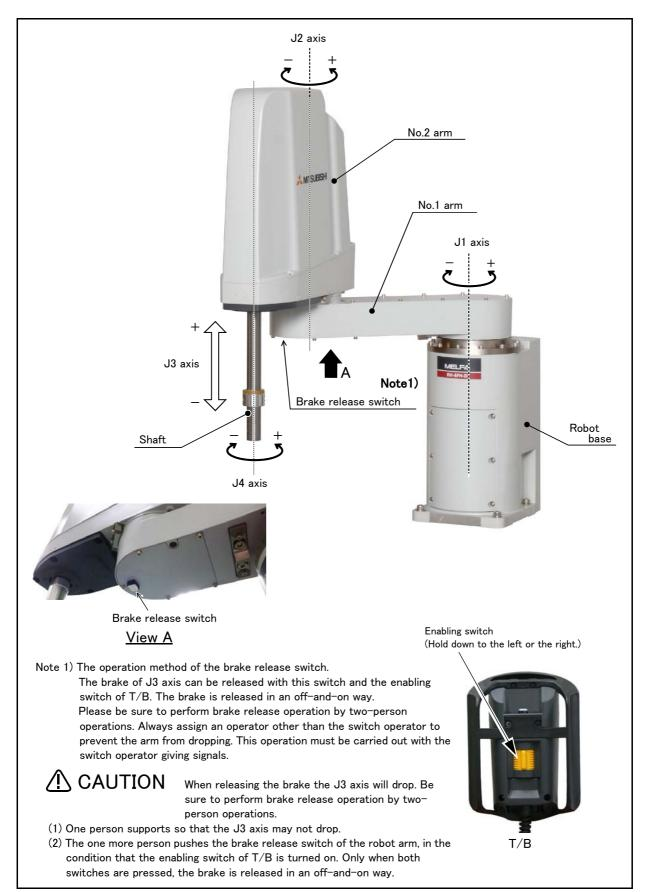
Fig.2-11: Names of each part of the robot
