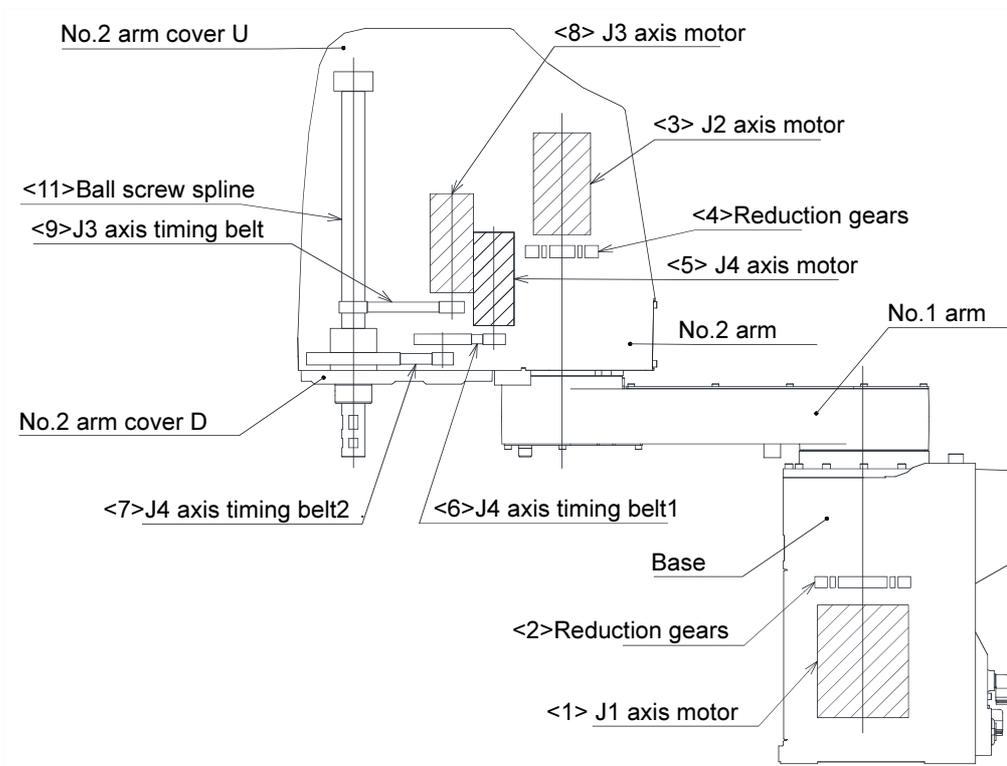
Fig.5-2 : Outline structure drawing of robot arm (RH-3FH)
