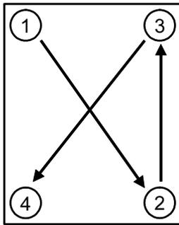
Fig.5-9 : Example of order which tighten bolts
