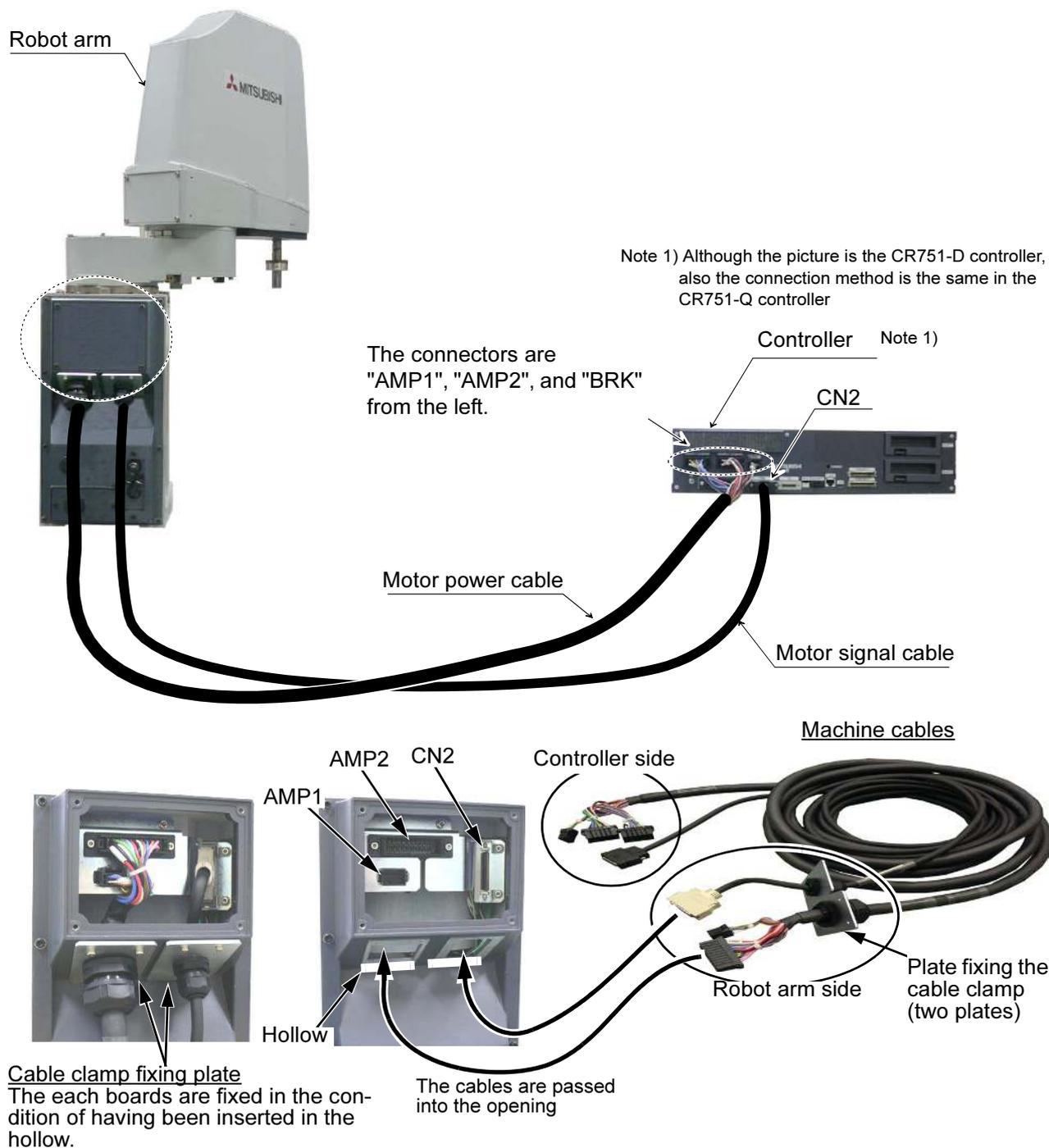
Fig.2-7 : Connecting the machine cables (RH-3FH, No-CE specification)
