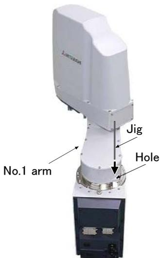
2) Move the J1 axis slowly toward the front using both hands. Align the pinhole of the No.1 arm and the pinhole at the base section, feed through the origin jig into the pinholes and fasten.
