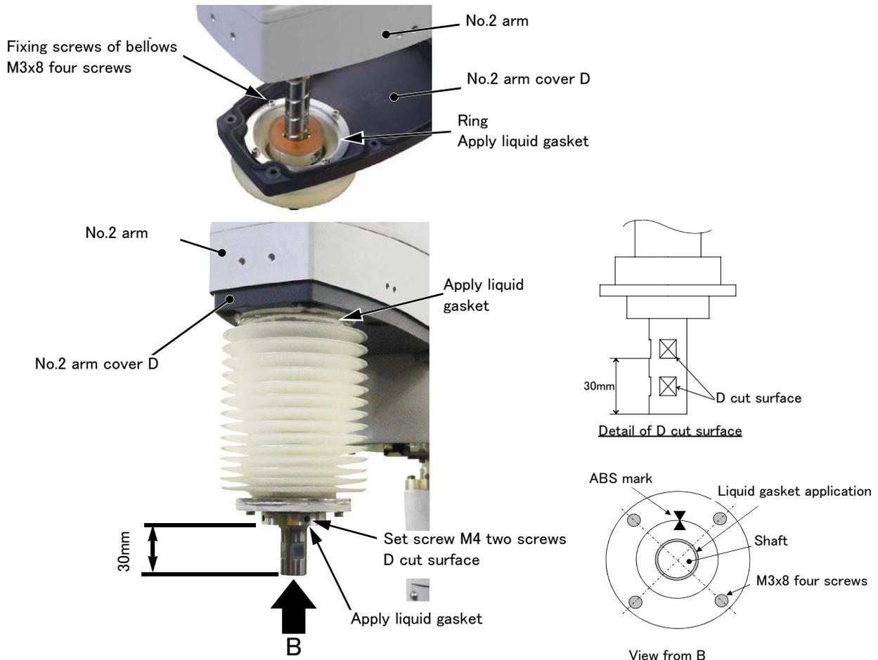
Fig.5-15 : Replace the bellows (clean specification)
