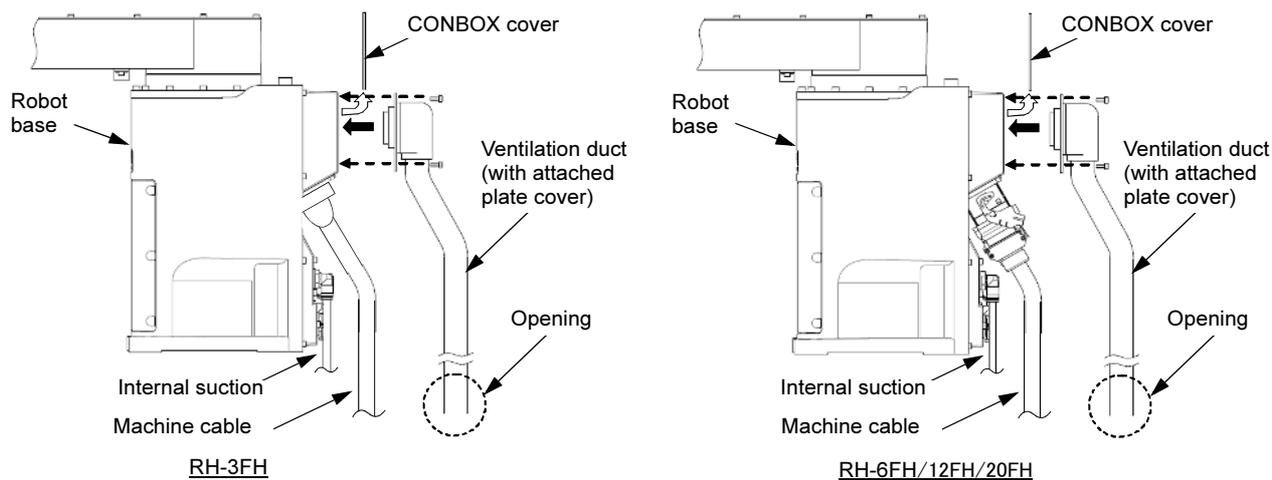
Fig.2-13 : Installation of Exhaust Duct
