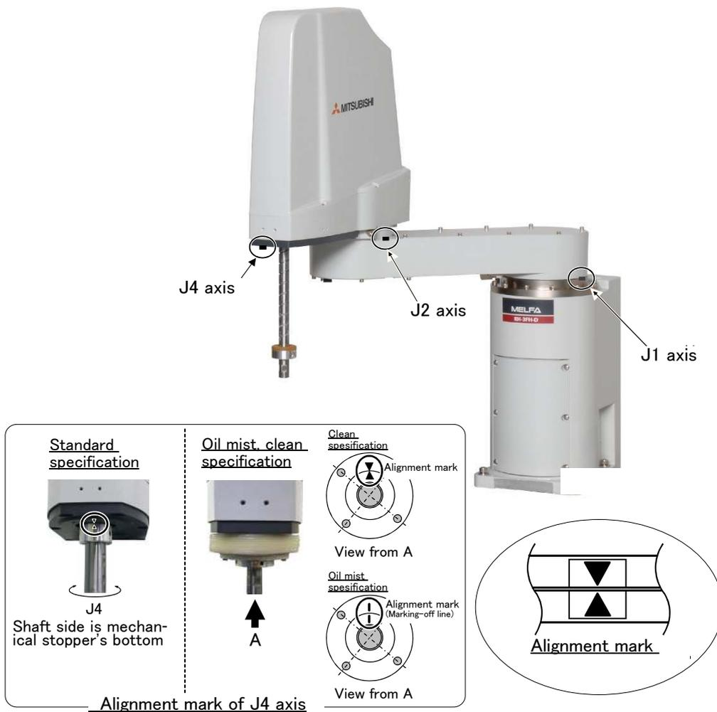
Note) There is no alignment mark of the J3 axis. Contact the J3 axis against mechanical stopper as the mechanism stopper method.
