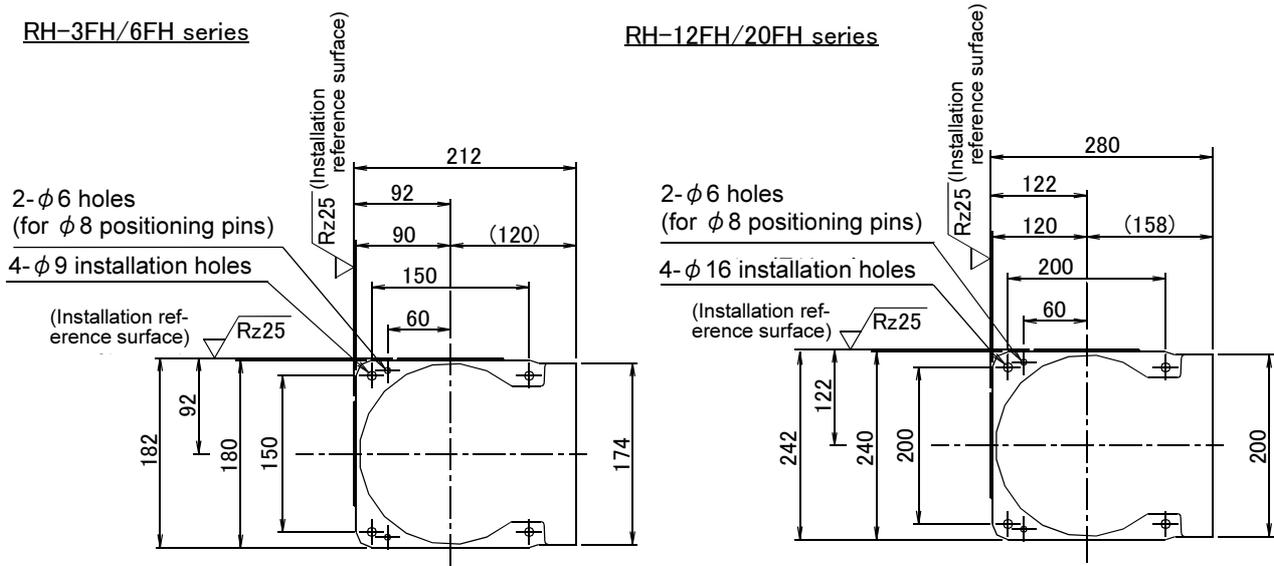
Fig.2-4 : Installation dimensions
