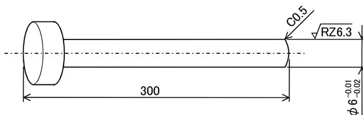
Fig.5-20 : Reference dimension of origin setting tool
