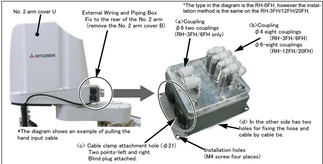
Table 3-2 : Hose and cables which can be pulled out
