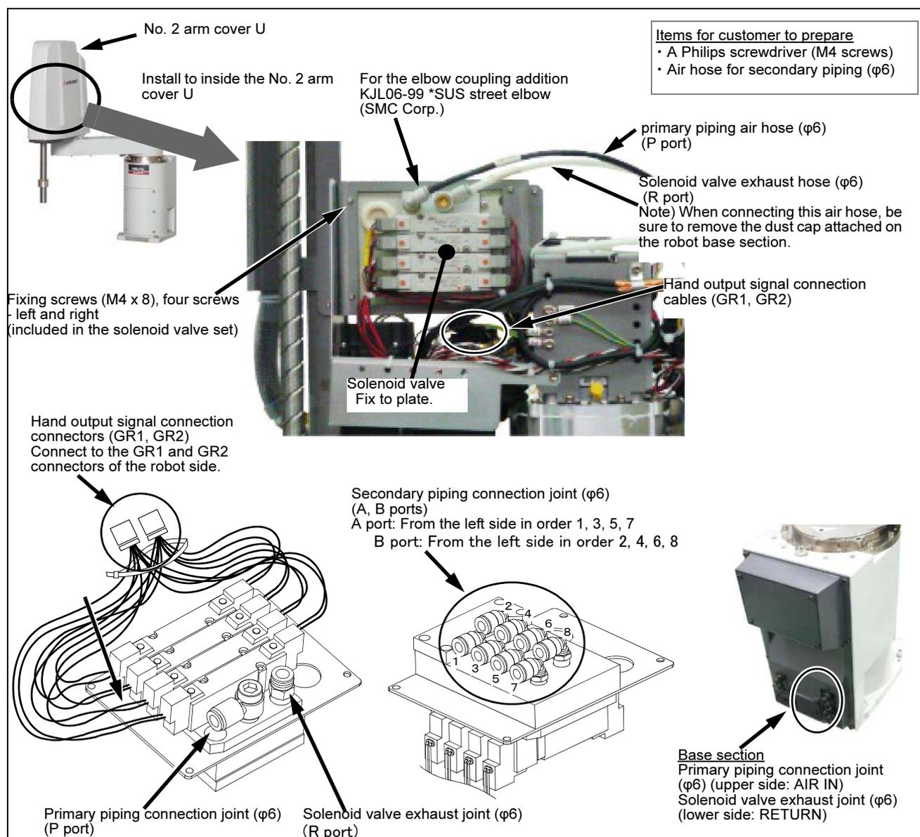
Fig.3-2 : Solenoid valve installation procedures (RH-12FH/20FH)
