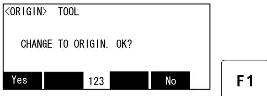
7) Press the [F1] key, and the origin position is set up.
