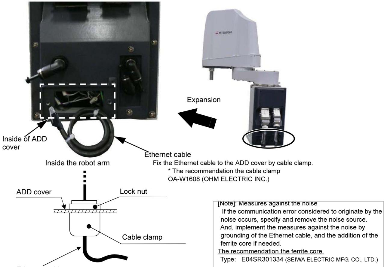
Fig.2-10 : Pull out the Ethernet cable (Base side)
