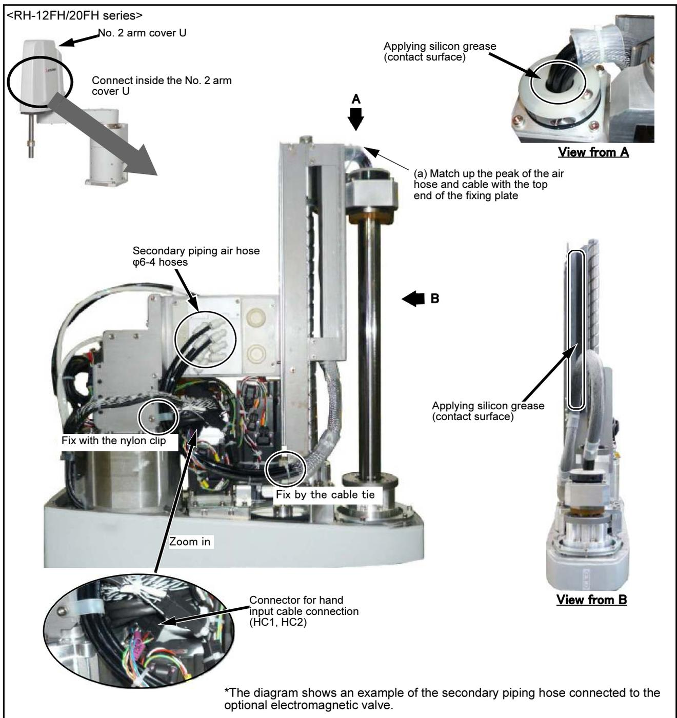
Fig.3-7 : Installing the hand internal wiring and piping set (RH-12FH/20FH)
