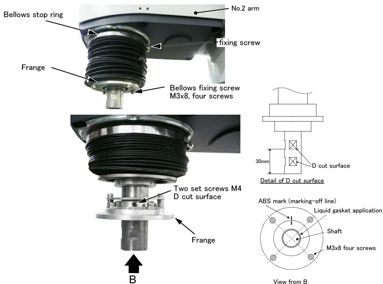
Fig.5-16 : Replace the bellows (oil mist specification)
