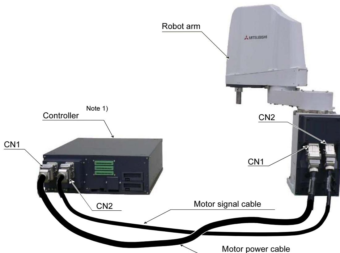
Note 1) Although the picture is the CR750-D controller, also the connection method is the same in the CR750-Q controller
