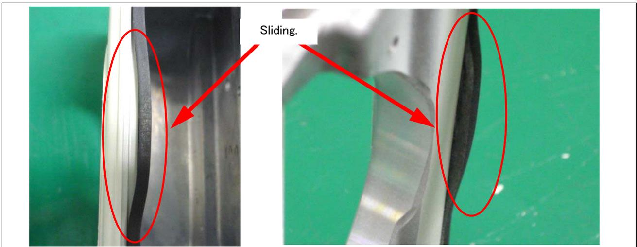
Fig.5-6 : Example of sticking packing (bad example)
