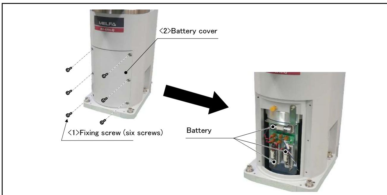
Fig.5-18 : Replacing the battery
