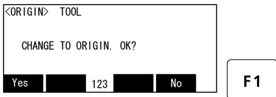
7) Press the [F1] key, and the origin position is set up.
