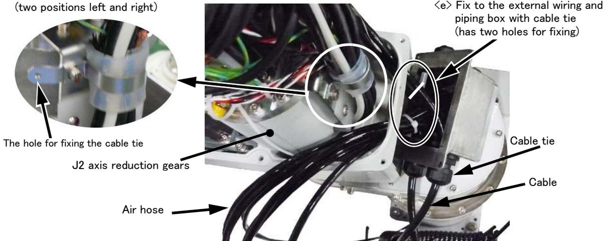
\*Diagram shows an image of pulling out air hose and cables
