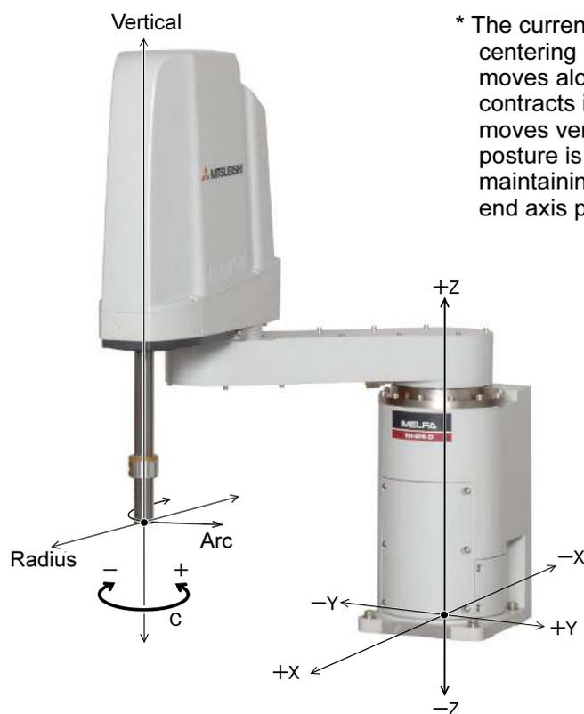
Fig.2-22 : CYLINDER jog operation
