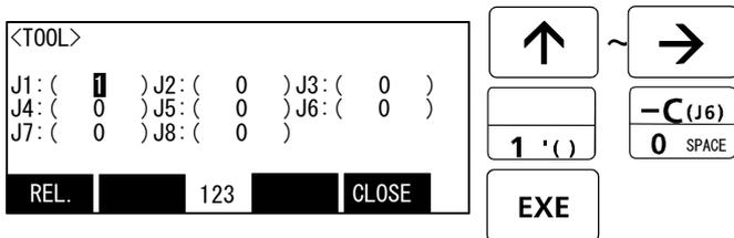
5) Input "1" into the J1 axis. Set "0" to other axes.
