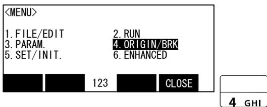
1) Press the [4] key on the menu screen, and display the Origin/Break selection screen.
