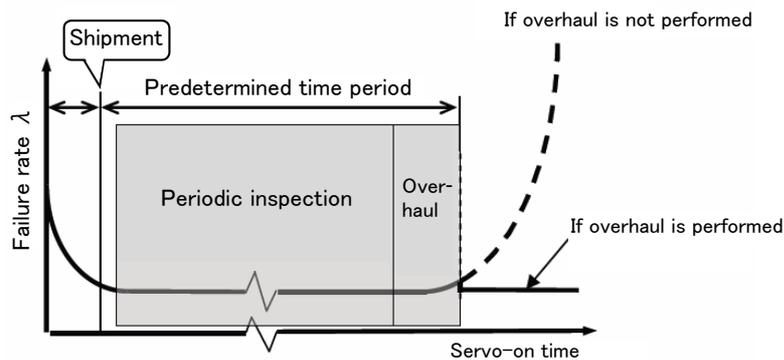
Fig.5-19 : Periodic inspection/overhaul periods
