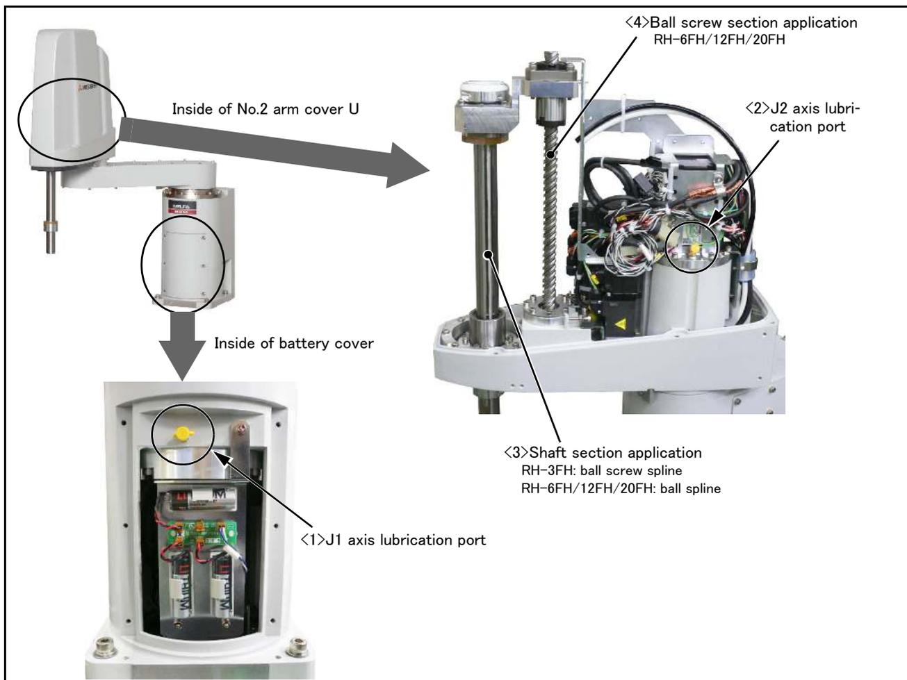
Fig.5-17 : Lubrication positions
