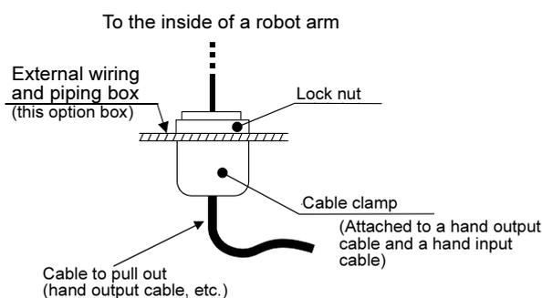
Fig.3-9 : Fixing the Cable
