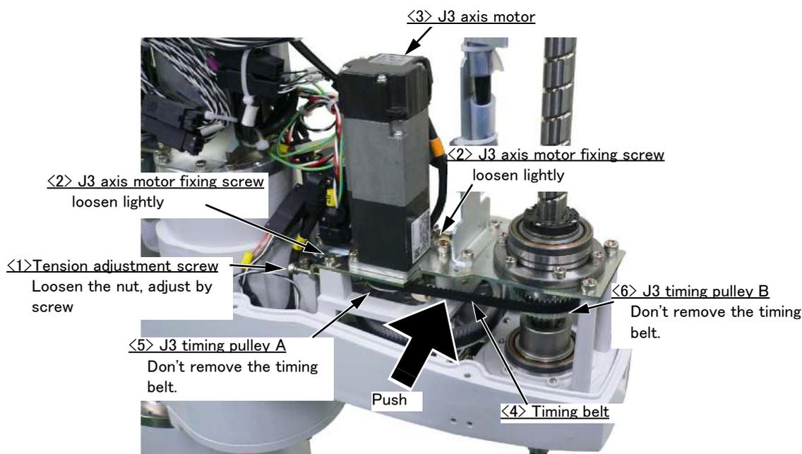
Fig.5-11 : Inspecting/Adjusting the J3 axis timing belt
