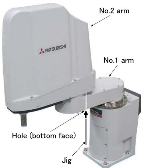
2) Slowly rotate the J2 axis 90° clockwise with both hands for RH-6FH series. Slowly rotate. Align the pinholes of the No. 1 and No. 2 arms, feed through the origin jig into the pinholes and fasten.
