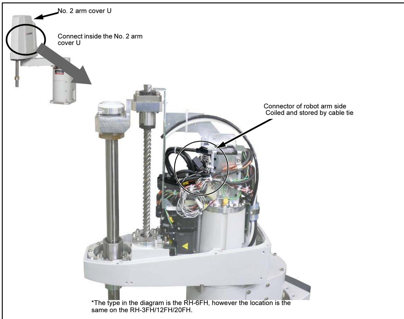
Fig.3-4 : Installing the hand output cable
