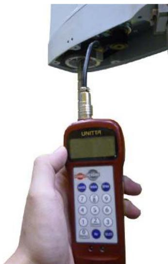
Measurement by the sound wave type belt tension gauge
