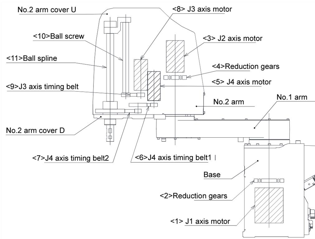
Fig.5-3 : Outline structure drawing of robot arm (RH-6FH/12FH/20FH)
