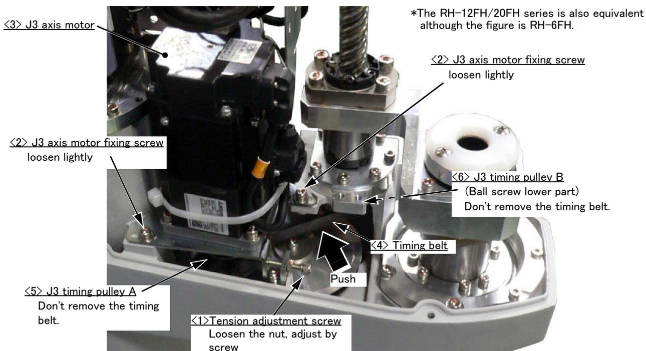
Fig.5-12 : Inspecting/Adjusting the J3 axis timing belt (RH-6FH/12FH/20FH)
