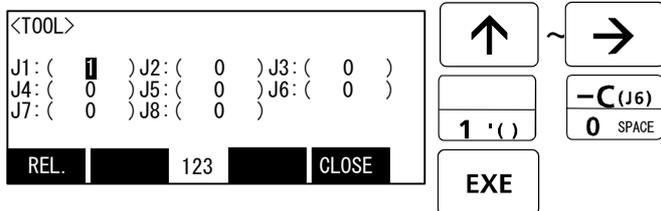
5) Input "1" into the J2 axis. Set "0" to other axes.
