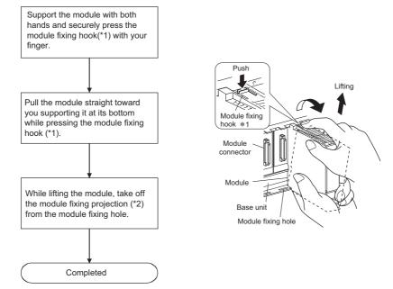
\*1 If the module has two module fixing hooks on its top, push the two modules fixing hooks on the right and left of the module top simultaneously with your fingers until they stop.
