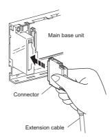
**4.** After fitting the extension cable, always tighten the extension cable connector fixing screws. (Tightening torque: 0.20N·m)
