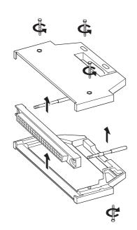
**1.** Loosen the four fixing screws on the connector and remove the screws. Open the connector cover from the connector side.
