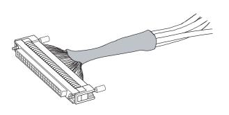
**1.** Check the terminal layout and press the wires against the connector.
