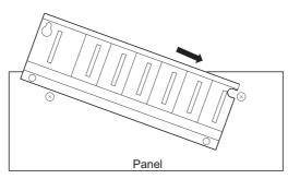
**3.** Place the left-hand side pear-shaped hole onto the left-hand side screw.
