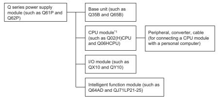
\*1 The CPU module is mounted on the main base unit.
