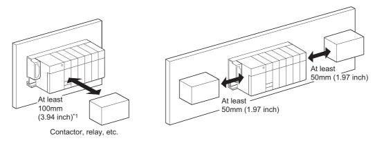
\*1 When using a Redundant CPU, keep a distance of 100mm (3.94 inches) or more between the programmable controller and the tracking cable.
