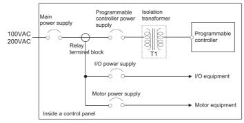
• If there is much noise, such as lightning surge, connect an isolation transformer. For details on the isolation transformer, refer to the following.
