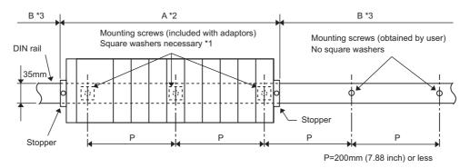
For Q00JCPU, Q00UJCPU, Q33B, Q35B, Q35DB, Q65B, Q52B, Q55B, Q63B, Q32SB, Q33SB or Q35SB type
