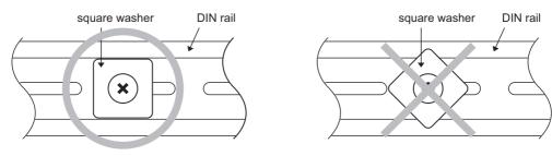
• Use the DIN rail that is compatible with M5 size screws.
