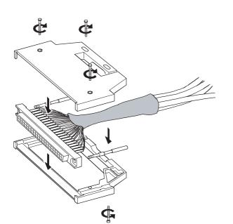
**4.** Place the connector on one side of the connector cover and put the fixing screws through the screw holes. Cover the other connector cover onto the connector.
