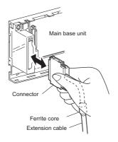
Holding the ferrite core may cause the cable disconnection in the connector.
