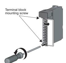
**1.** Open the terminal cover and loosen the terminal block mounting screw.
