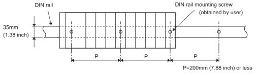
When installing the DIN rail in a frequent vibration and/or shock prone environment, insert the mounting screws in 200mm intervals or less by the following method show below.
