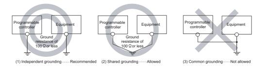
• Use thick cables up to 2mm<sup>2</sup>. Bring the grounding point close to the programmable controller as much as possible so that the ground cable can be shortened.
