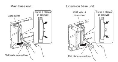
2. To connect the extension cable to the next extension base unit, remove the seal put under the IN characters on the base cover.
