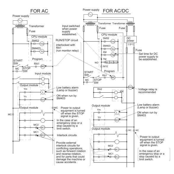
The power-on procedure is as follows: For AC
