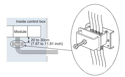
The AD75CK enables up to four cables to be grounded together if the outside diameter of the shielded cable is about 7mm.
