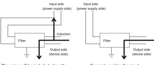
The noise will be included when the input and output wires are bundled.
