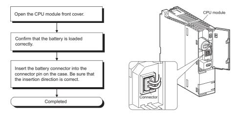
(b) High Performance model QCPU, Process CPU, Redundant CPU and Universal model QCPU
