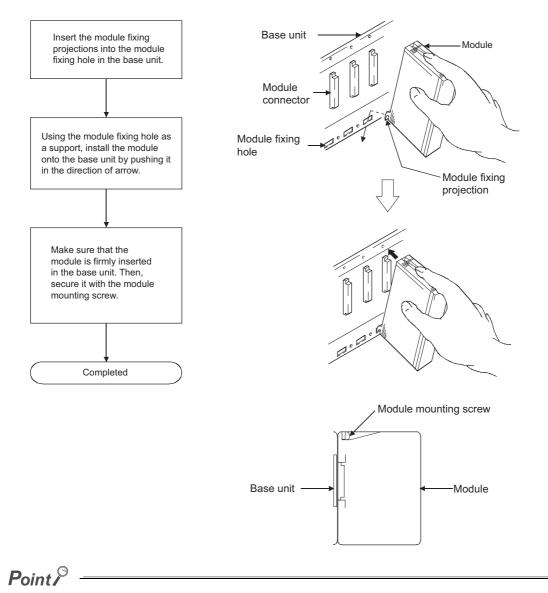
Make sure to mount the module with the module fixing projection inserted into the module fixing hole, using the module mounting screws.
