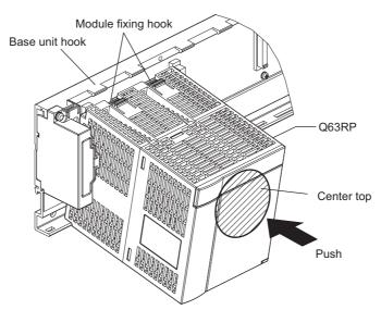
\*2 If the module has two module fixing hooks on its top, push the center top of the module so that the two module fixing hooks on the right and left are securely engaged with the base unit hooks.
