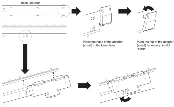
Insert the adaptor (large) into the grooves of the base unit from below.
