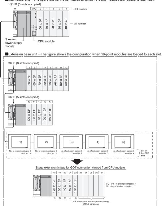
Main base unit ... The figure shows the configuration when 16-point modules are loaded to each slot.
