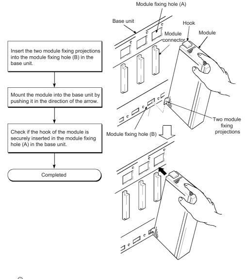
4.2 Module Installation 4.2.3 Installation and removal of module
