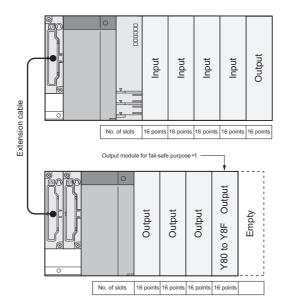
\*1 The output module for fail-safe purpose must be mounted in the last slot of the system. (Y80 to Y8F in the above system.)
