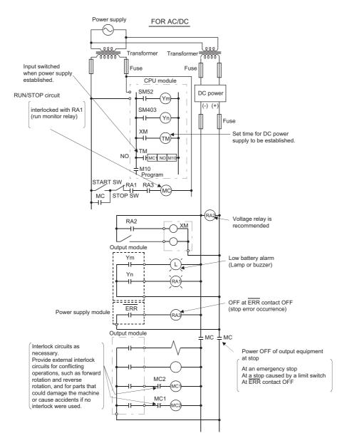
The power-on procedure is as follows: For AC/DC
