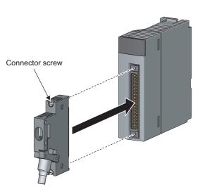
**1.** Plug the connector into the slot on the module.
