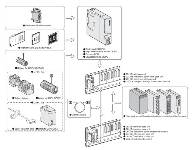
The combination of modules depends on the devices used in the configuration.
