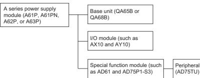
Select the power supply module also in consideration of the current consumption of the peripheral devices connected to the special function module.
