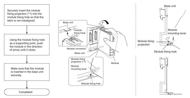
\*1 If the module has two module fixing projections, insert the two module fixing projections on the right and left into the module fixing holes so that they are not misaligned.
