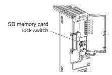
When removing the SD memory card while the power is on, check that the SD CARD LED is off.
