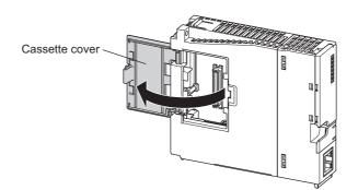
2. Hold the top and the bottom of the knob of the extended SRAM cassette, and insert it straight into the cassette connector.
