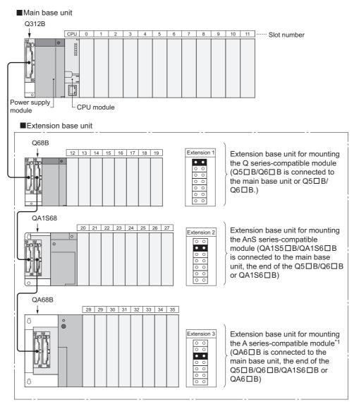
\*1 When using the QA6ADP+A5 $\Box$ B/A6 $\Box$ B, connect it below the QA6 $\Box$ B.
