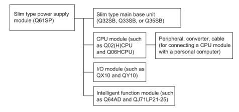
Keep the current consumption of the slim type main base unit (Q3□SB) not exceeding the 5VDC rated output current of the slim type power supply module (Q61SP).
