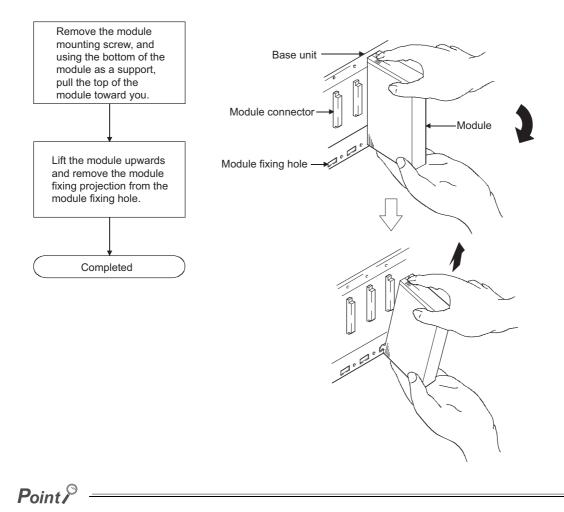
When removing the module which is secured by module mounting screw, remove the module mounting screw first and then module fixing projection off the module fixing hole of the base unit. Failure to do so may damage the module fixing projection.
