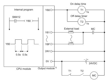
\*2 Y80 repeats turning on and then off at 0.5s intervals. Use a no-contact output module (transistor in the example shown above).
