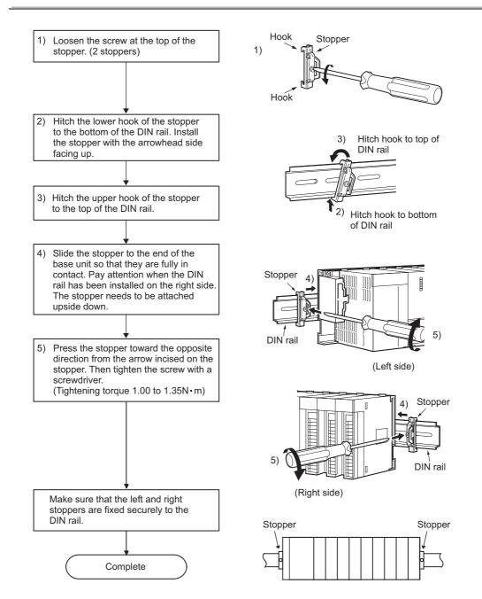
In addition, when three or more modules with 130mm or more in depth (such as Q66DA-G etc.) are mounted, or when the base unit is used in the environment with extremely frequent vibration, use the Q6DIN1A Q-type base DIN rail mounting adaptor (vibration-proofing bracket kit) where the large mounting bracket is included. The large mounting bracket enables to enhance the resistance to vibration. Depending on the environment, it is recommended to mount the base unit directly on the control panel.
