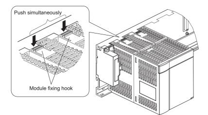
\*2 If the module has two module fixing projections, remove the two module fixing projections on the right and left of the module bottom from the module fixing holes.
