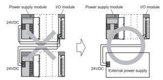
• 100VAC, 200VAC and 24VDC wires must be twisted as dense as possible. Connect the modules with the shortest distance.
