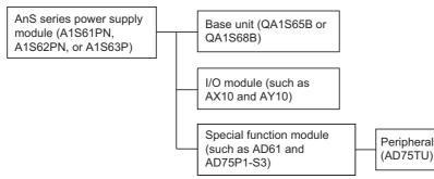
Select the power supply module also in consideration of the current consumption of the peripheral devices connected to the special function module.
