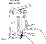
**3.** When plugging the extension cable to any base unit, hold the connector part of the extension cable.
