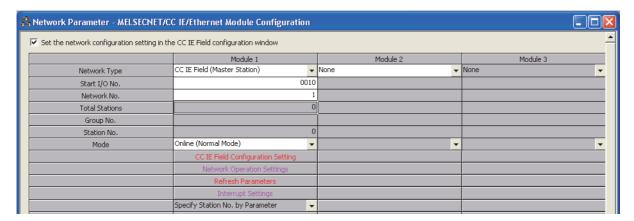
3. Open the network configuration setting window and set parameters as follows.
