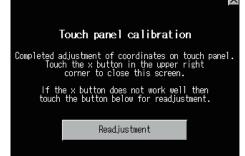
5. Touching the X button displayed on the upper right returns the screen to the previous screen. When the precise touch could not be made, touch the [Readjustment] button to make the setting from again.
