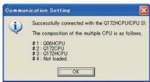
Confirm that the PC is connected to the motion controller CPU (Q series).
