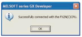
The screen returns to the [Transfer Setup]. Click the Connection Test to check if GX Developer has been connected to the FXCPU.
