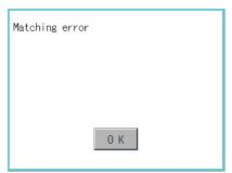
If selected record does not match to the device value of controller, the dialog box shown left is displayed.
