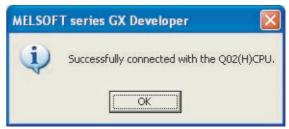
The screen returns to [Transfer Setup]. Click Connection Test to check if GX Developer has been connected to the QCPU (Q mode).  Connecting the GOT and PLC in computer link connection (when connecting to QJ71C24(N))
