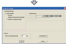
Mark the [Serial port/USB] checkbox in [Connecting interface].
