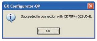
The screen returns to the [Transfer setup]. Click the Connection Test to check if GX Developer has been connected to the QD75\*\*\* (QnCPU).
