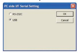
4. Double-click [Serial] of the PC side I/F to display [PC side I/F Serial setting].
