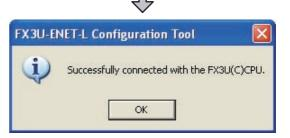
The communication test is executed. Check that the GOT is correctly connected to the FXCPU.
