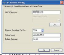
\*3 Each of [GOT PLC No.] set in the communication detail setting and [PLC No.] set in the Ethernet setting must be set to different station numbers.
