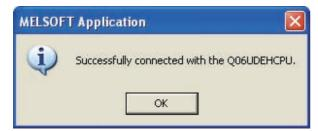
15. The screen returns to [Transfer Setup]. Click Connection Test to check if GX Developer has been connected to the QCPU (Q mode).
