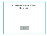
When the connecting target confirmation communication ends, its result is notified by dialog box. If the connecting target confirmation communication ends normally, the dialog box notifying of the normal termination mentioned left is displayed. Touching [OK] button after confirming the result returns to [I/O check].
