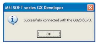
The screen returns to [Transfer Setup]. Click Connection Test to check if GX Developer has been connected to the QCPU (Q mode).  Connecting the GOT and PLC in Ethernet connection (when connecting to QCPU (Q mode))
