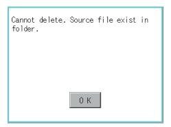
4. When it cannot be deleted, the dialog box shown at left appears. (Only when deleting folder is executed.)
