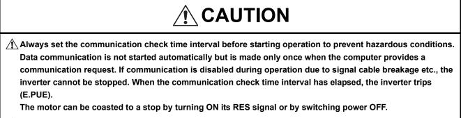
If communication is broken due to signal cable breakage, computer fault, etc, the inverter does not detect such a fault. This should be fully noted.
