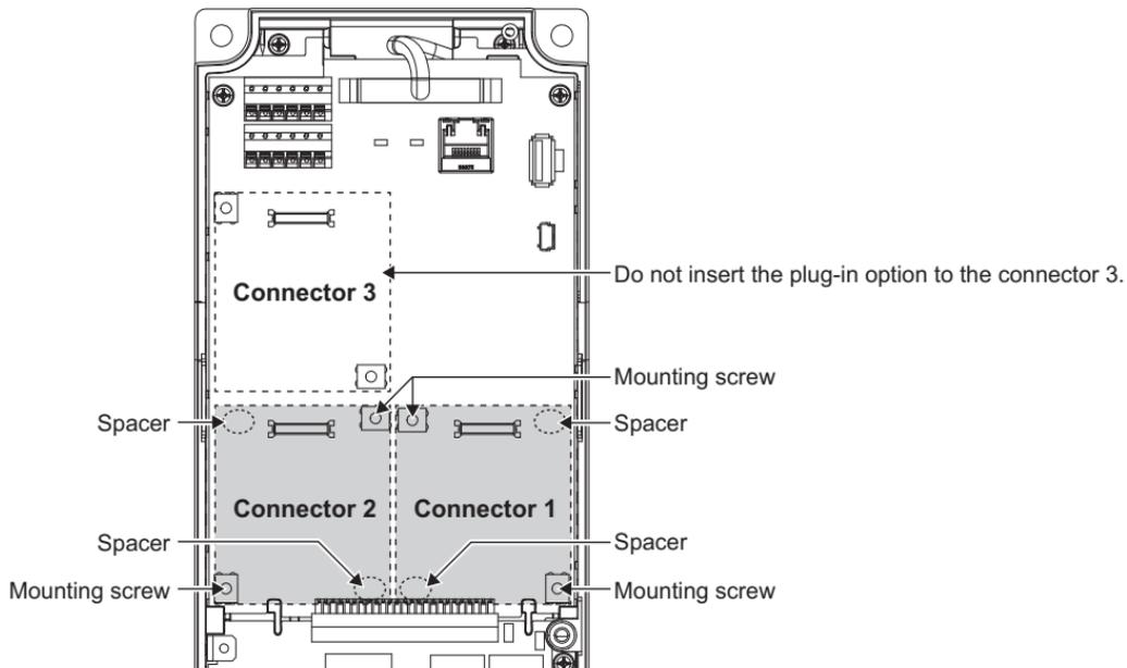
**Insertion positions for screws and spacers**
