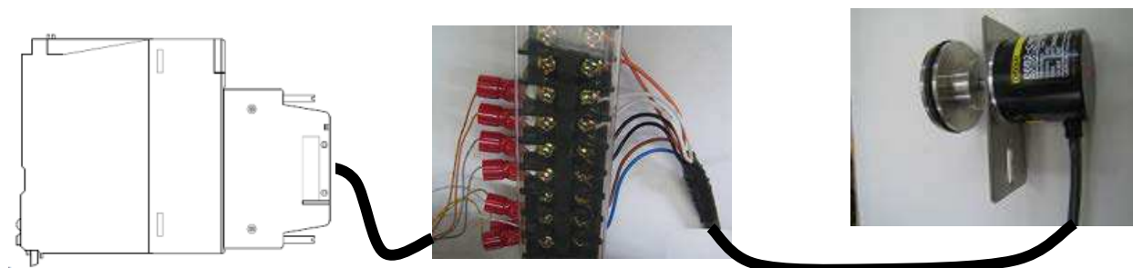
Figure 5-7 Wiring example (CR75x-Q/ CRnQ-700 series controller)
