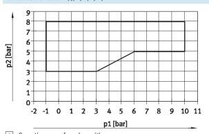
1 Operating range for valves with external pilot air supply
