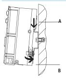
The MPA valve terminal is attached to the H-rail (see arrow A).
