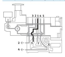
The reversible B regulator splits the supply air in duct 1 and regulates the pressure upstream of the valve in duct 3 (the unregulated pressure from duct 1 is in duct 5). The regulated air is then supplied to duct 2. The valve is thus operated in reversible mode.
