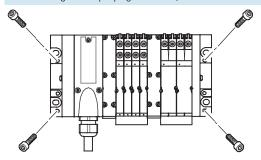
The MPA valve terminal is screwed onto the mounting surface using four M4 or M6 screws. The mounting holes are on the pneumatic interface and on the right-hand end plate. There are also optional mounting brackets available.
