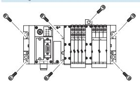
The MPA valve terminal is screwed onto the mounting surface using six M4 or M6 screws. The mounting holes are on the left-hand end plate (CPX) and on the right-hand end plate MPA.
