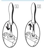
1 Press in the stem of the MO with a pin or screwdriver. Pilot valve switches and actuates the main valve.
