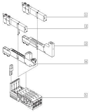
Vertical stacking components, MPA2
