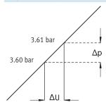
The response sensitivity of the device determines how sensitively one can change, i.e. adjust, a pressure.
