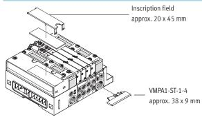
An inscription label holder VMPA1-ST-1-4 (Part No. 533 362, code T in the order code) or VMPA1-ST-2-4 (Part No. 544 384, for holding IBS-6x10 inscription labels) can be mounted on each manifold block with a width of 42 mm for labelling the valves.
