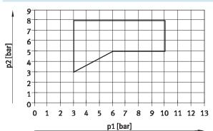
① Operating range for valves with external pilot air supply
