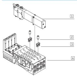
The fixed restrictor can be used to permanently set the flow rate in ducts 3 and 5 when exhausting air. To be able to screw the restrictor into the sub-base, the retainer is first pressed as far as it will go into the exhaust openings on the sub-base.
