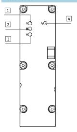
The pressure sensor indicates whether the applied pressure exceeds, adheres to or falls below the setpoint value using three LEDs. An additional LED indicates common errors (limit exceeded or fallen below).
