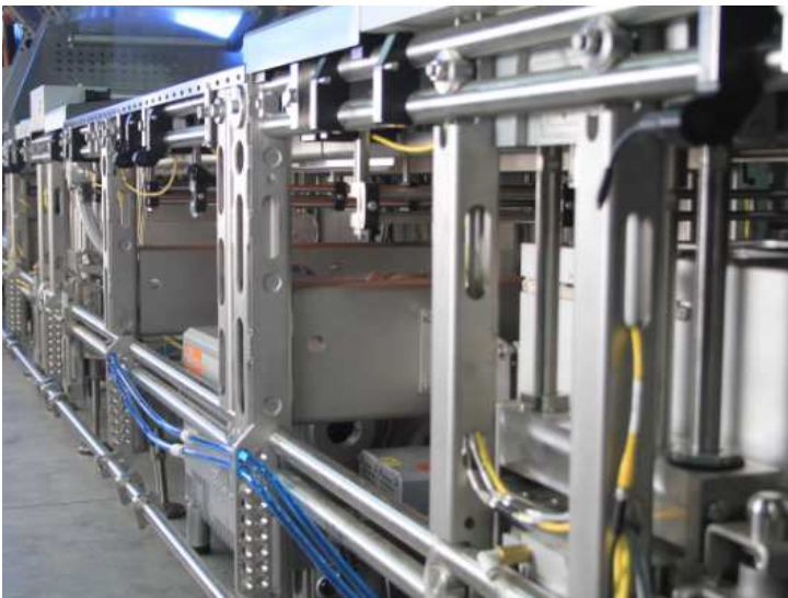
The i-Series High Performance Thermoformer from VC999 Packaging Systems is powered by Mitsubishi Electric's L Series PLC and utilizes the 1 Gbps Ethernet-based CC-Link IE Field industrial network.
