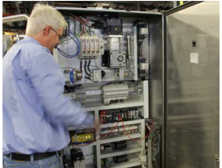
The i-Series High Performance Thermoformer from VC999 Packaging Systems is powered by Mitsubishi Electric's L Series PLC and utilizes the 1 Gbps Ethernet-based CC-Link IE Field industrial network.
