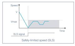
Function to monitor the speed so that the predetermined speed limit is not exceeded.
