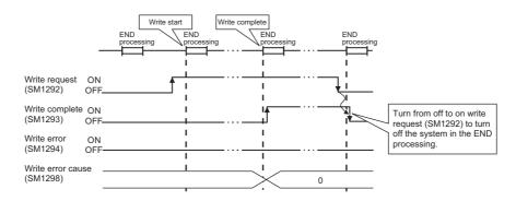
(b) Operations of special relay and special register when the operation of writing to the IP address storage area (flash ROM) failed
