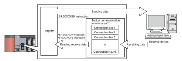
The area is used for storing data received from the connected open devices.
