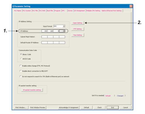
1. Set the IP address of the CPU module.
