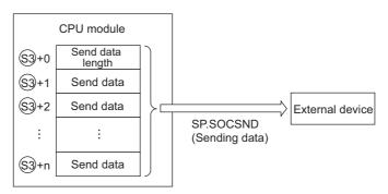
The result of the SP.SOCSND instruction can be checked with the completion device, ©+0 and ©+1.
