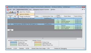
6. Write the protocol setting data to the CPU module. In the "Writing Protocol Setting" window, specify the write-target drive in the CPU module and write the
