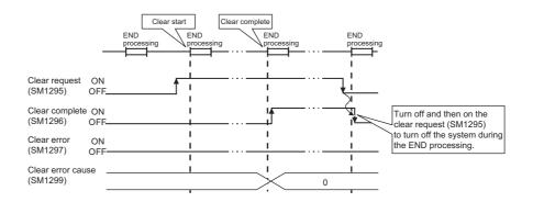
(b) Operations of special relay and special register when the operation of clearing the IP address storage area (flash ROM) failed
