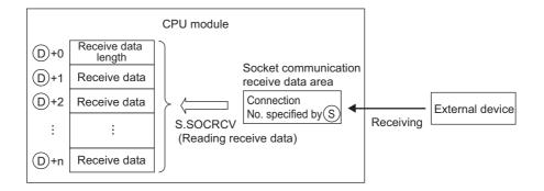
The following figure shows the timing of reception processing with the S.SOCRCVS instruction.
