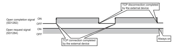
When a device establishes a connection by Passive open, the IP address and port number of the connected device can be acquired using the SP.SOCCINF instruction.
