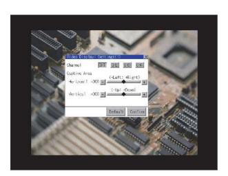
The captive area (horizontal direction/vertical direction) for the selected channel No. can be changed.
