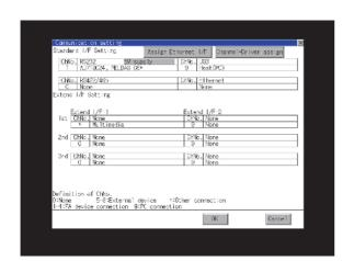
Install communication driver [Q/L/QnA/A CPU, QJ71C24, LJ71C24] to GOT.
