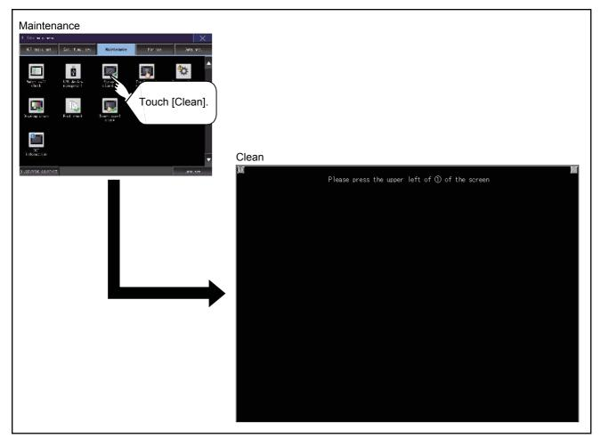
Even if touch points other than the upper left corner and upper right corner of the screen, the GOT does not operates.
