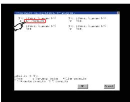
Touch the driver display BOX of the communication parameter to be set in the [Ethernet I/F assignment] screen.
