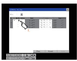
Touch the Net No. to be changed, and input the network No. to be changed by the numeric keypad displayed.
