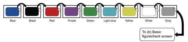
If touch the upper right part of the screen at the final color (white screen), the following 2) Basic figure check screen is displayed.
