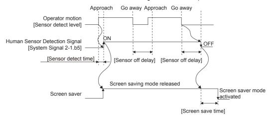
When there is no operator around the GOT for the time set as "Sensor OFF delay", the "Human Sensor Detection Signal" turns OFF.
