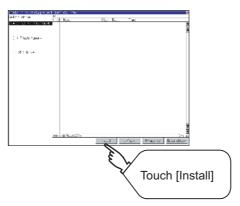
The USB memory access LED is lit during install execution.Do not pull out the USB memory or power OFF the GOT while the USB memory access LED is lit.
