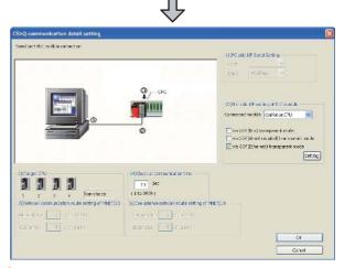
On the [PLC side I/F setting of PLC module], mark the [via GOT (Ethernet) transparent mode] checkbox and click [Set].
