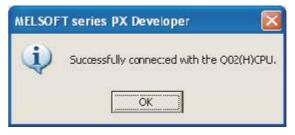
The screen returns to [Transfer Setup]. Click [Connection Test] to check if PX Developer has been connected to the QCPU (Q mode). Connecting the GOT and PLC in computer link connection(when connected to the QJ71C24(N)) (GX Configurator is not supported.)
