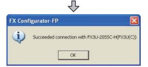
After the communication test is completed, check that the GOT is correctly connected to the FXCPU.
