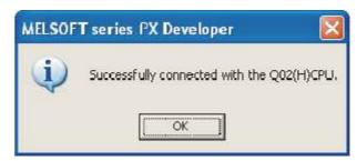
The screen returns to [Transfer Setup]. Click [Connection Test] to check if PX Developer has been connected to the QCPU (Q mode). When connecting the GOT and PLC in Ethernet communication (when connecting to QCPU (Q mode))
